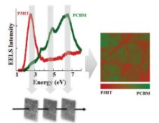
Monochromated transmission electron microscopes can generate contrast in organic thin films based on differences in the valence electronic structure at energy losses below 10 eV. By applying principal component analysis to the spectroscopic image series, further details about phase compositions and local electronic transitions in the active layer of organic semiconductor mixtures can be explored.
